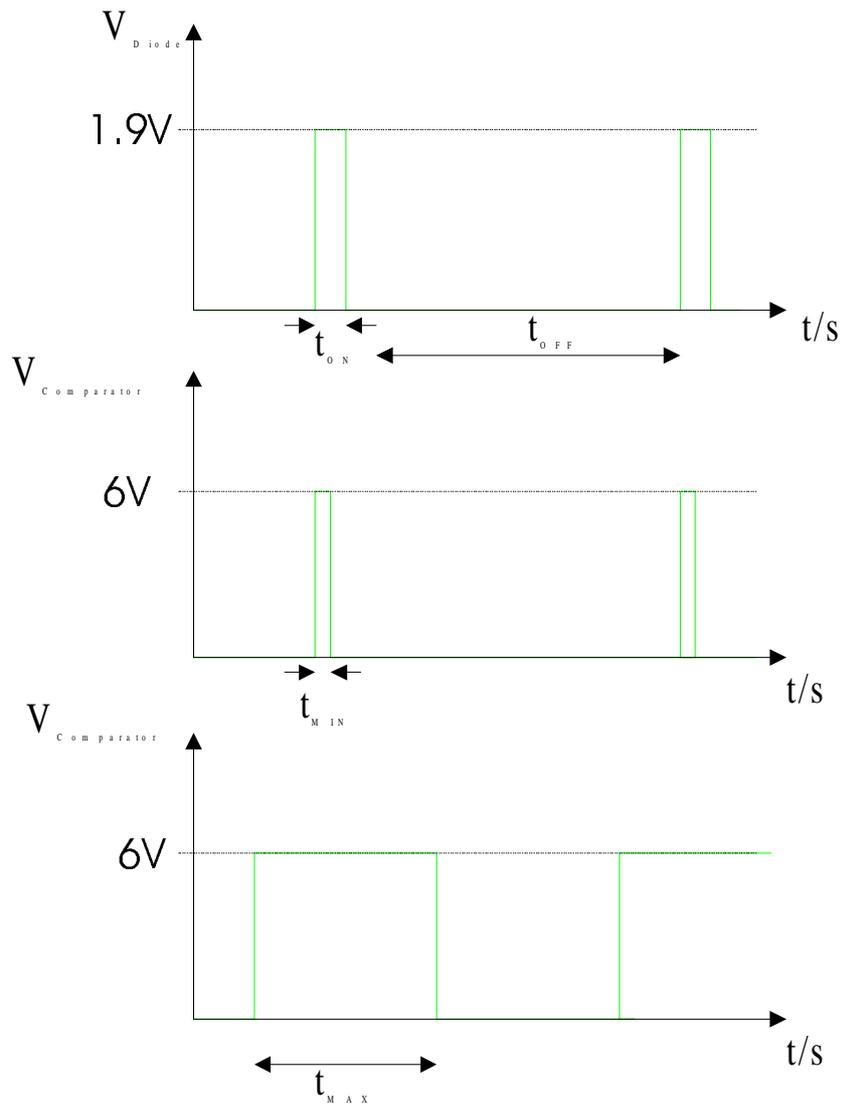
**figure 6 - Diode Voltage and Comparator Output**
