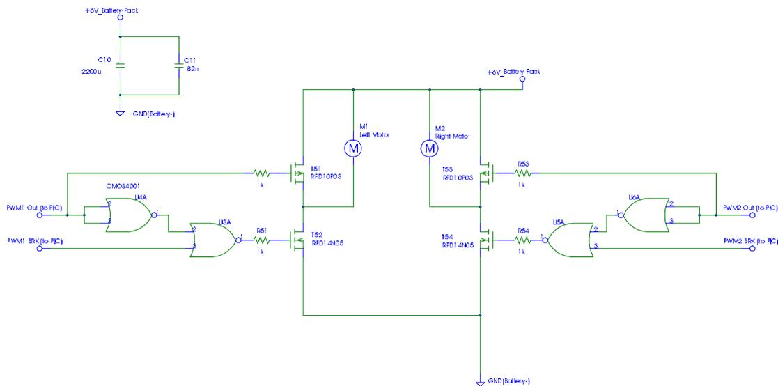
**figure 10 – Motor driver stage (power stage)**
