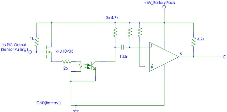
**figure 5 – Schematics of one Sensor-stage**
