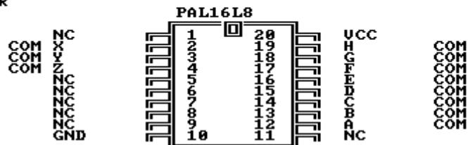
The pinout is directly derived from the declaration segment in the listing and every change in the listing appears in the pinout view.
