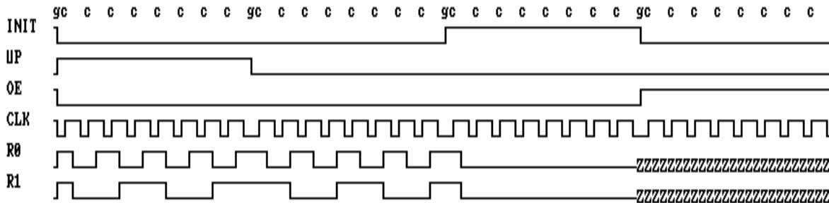
A comparision between the truth table and the waveform shows the correct working of the counter. An automatic check of the software was here not programmed, because it would be very complex, and errors can occur very easily.
