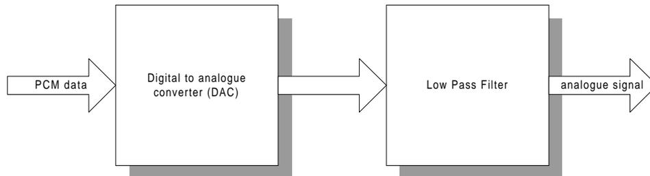
The quality of the reconstructed signal is at all depending on the resolution and so on the number of different bits transmitted. Usually PCM systems work with 8 or 16 data bits.
