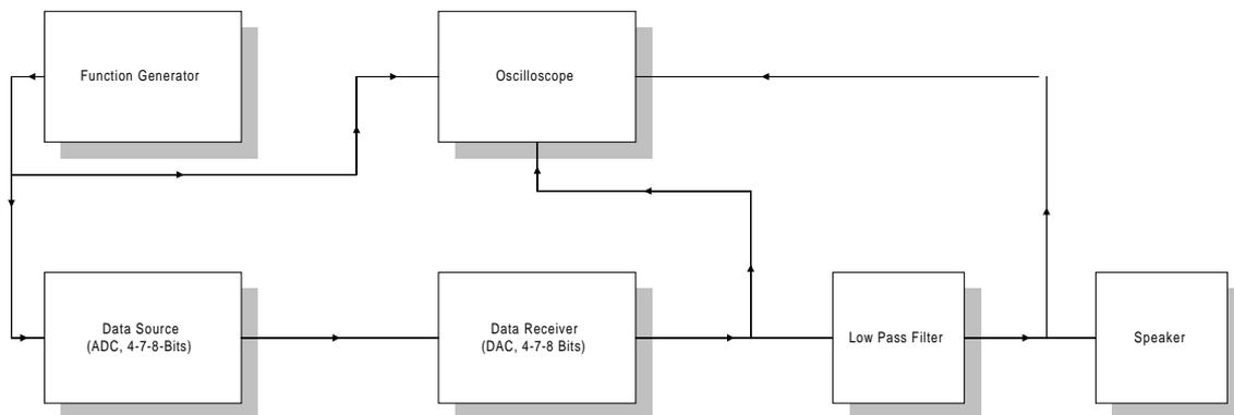
**figure 4 - block diagram**
