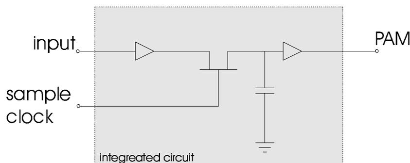
figure 2 – Sampling circuit
