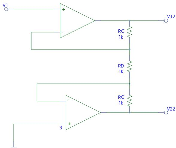
$$\frac{V_{21}}{V_1} = \frac{R_C + R_D}{R_D}$$
