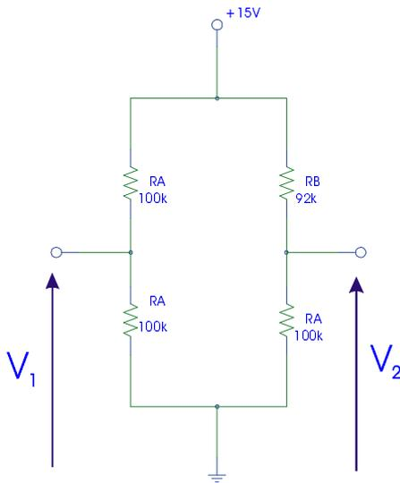
The bridge outputs were  $V_1=7.5\text{V}$  and  $V_2=7.67\text{V}$ .
