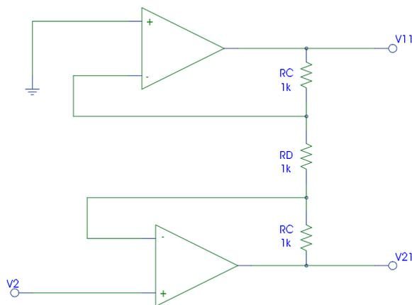
$$\frac{V_{21}}{V_2} = \frac{R_C + R_D}{R_D}$$
