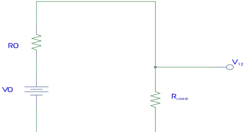
The output voltages of the bridge change when the bridge is connected to the opamp stage because the amplifier inputs are a load to the bridge. The new bridge output voltages can be calculated using Thevenin's theorem, where  $V_0$  is the disconnected bridge voltage.
