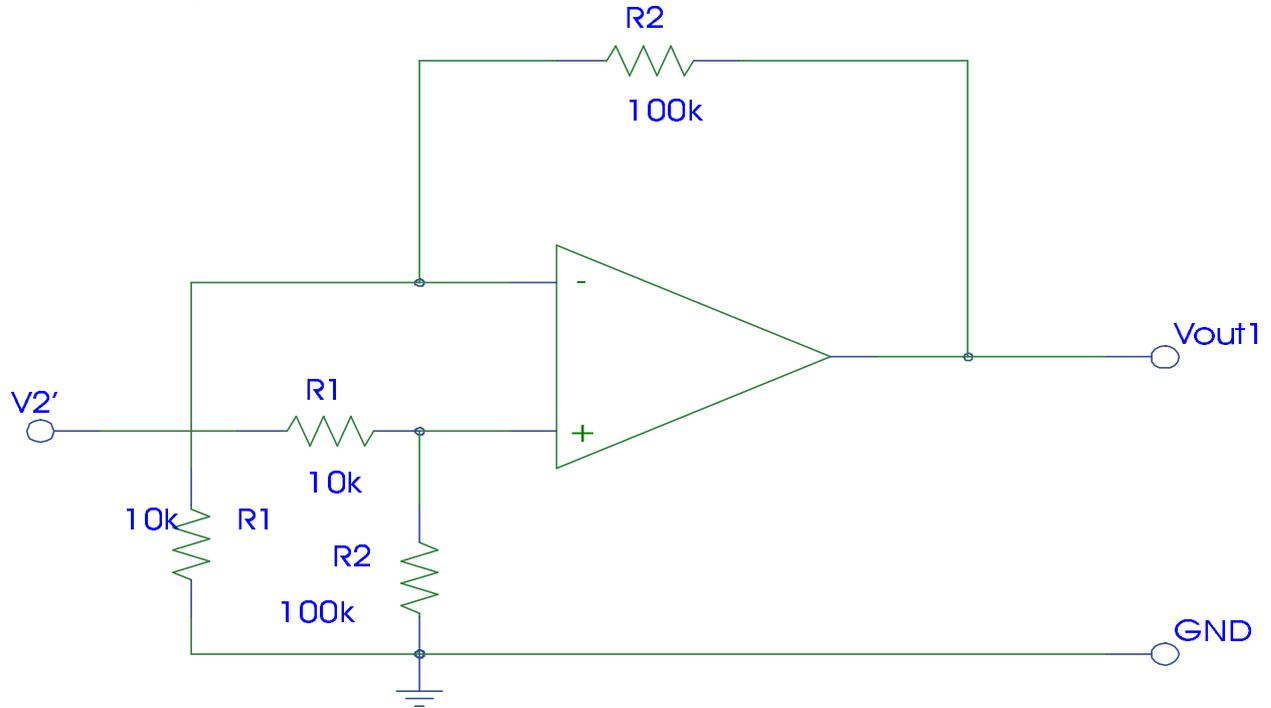
The output voltages of the connected bridge are now nearly the same than the output voltages of the unconnected bridge, because they are only connected to the opamp inputs which have an input resistance of more than several hundreds k $\Omega$  (for the LM741 typically 2M $\Omega$ ).
