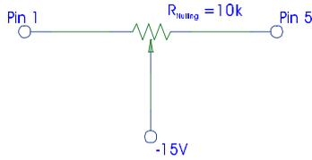
The above figure shows the connection of a nulling potentiometer to an opamp LM741, which was used in the Lab.
