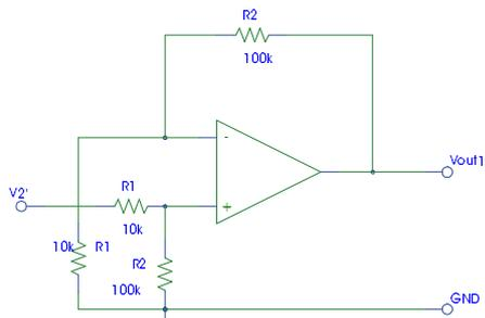
$$\frac{V_{\text{Out1}}}{V_+} = \frac{R_2 + R_1}{R_1} \rightarrow (V_1' = 0V)$$
