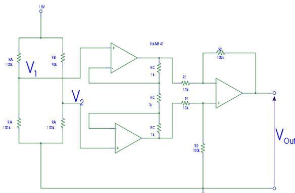
The output voltages of the bridge decrease when connecting to the opamp-circuit because of its load function.
