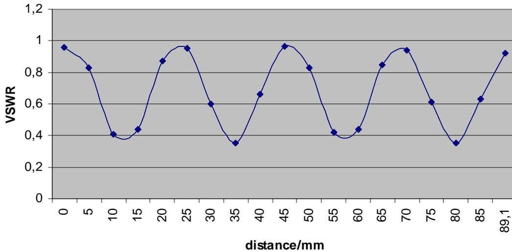
In the Lab not all of the energy was reflected (minimum VSWR=0.41), because some energy was absorbed on the open end.
