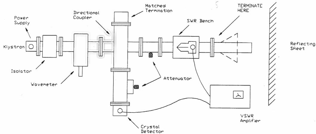
The lab equipment consists of a Klystron, as a microwave source, a directional coupler, an SWR Bench, a VSWR meter. Different terminations can be applied to the equipment, which were a matched termination, a short circuit and an open circuit and a matched horn aerial with reflector to measure the wavelength.
