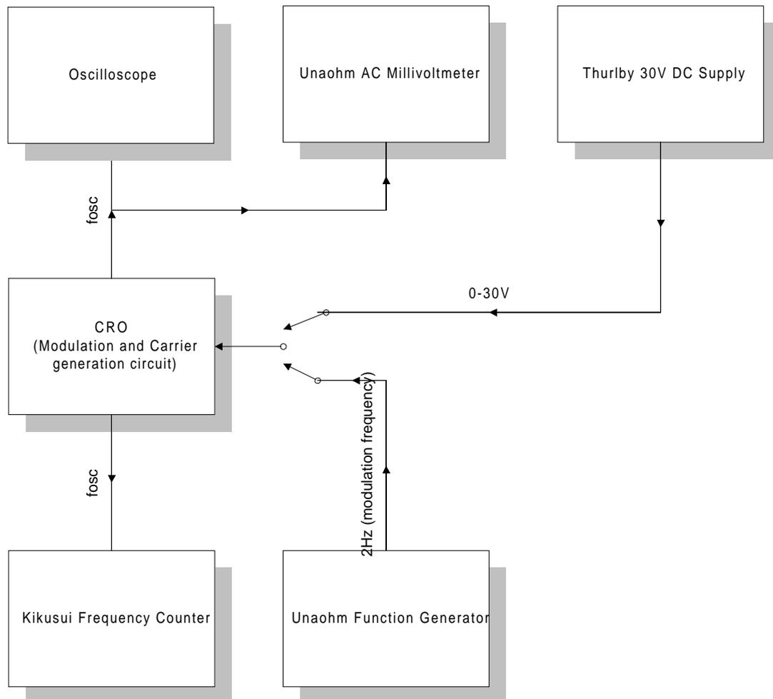
The CRO unit generates the carrier frequency and contains a built-in varicap diode and a calibrated capacitor with which the carrier frequency can be either manually or electronically changed by applying a voltage to the varicap. A Thurlby 30V DC power supply and a Unaohm frequency generator can generate an appropriate voltage therefore.
