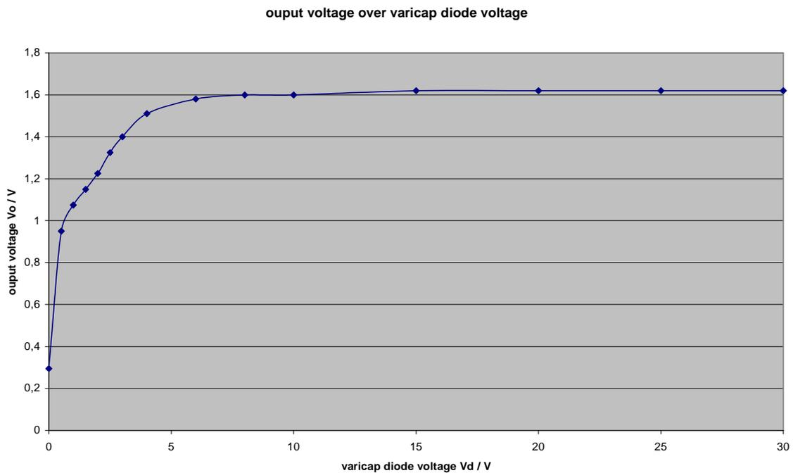
The output voltage is not at a stable level when only small voltages (low frequencies) are applied to the varicap. This results from the inner structure of the CRO.
