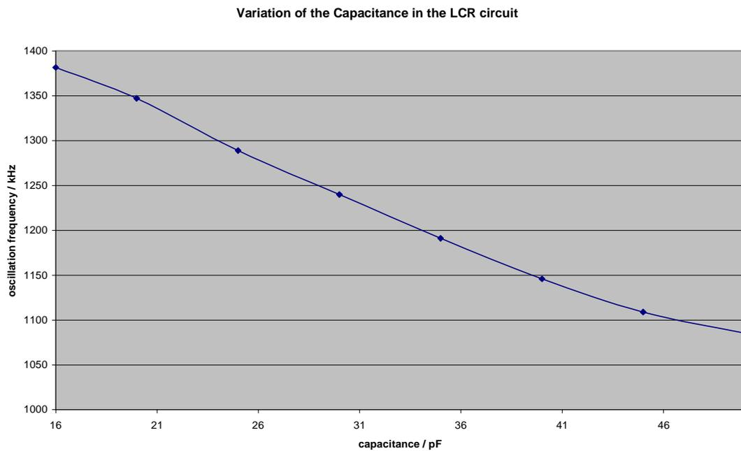
The variance of the capacitance  $C$  results in a nearly linear variance of the resonance frequency.
